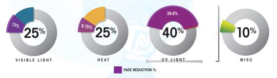
This helps me out tremendously I can now inform the customer that they can expect a 62% reduction in fading after the installation of Daylight Natural 50%. I continue to point out that the 10% miscellaneous cause of fading is a complete unknown. The steadfastness of the dye, the age of the furnishings and even humidity are beyond our control.
